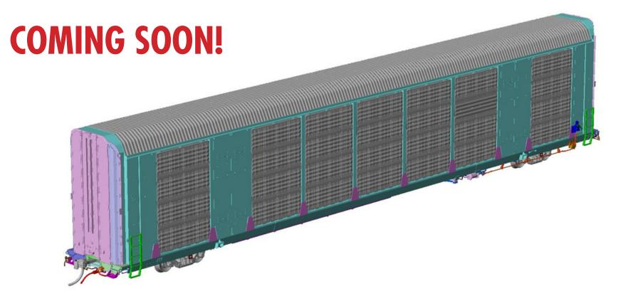
In 2013, Greenbrier Companies introduced their new design of 89' auto rack, the Multi-Max<sup>™</sup>. The new design allows for changing configurations from a Bi-Level to a Tri-Level (and back) without adding or removing decks. The racks are fully compatible with existing 89' auto racks. To this date, most of the racks have been built on Greenbrier Companies' own specially designed 89' flat cars. Currently, we're approaching 10,000 cars (with racks) running on North American rails.
