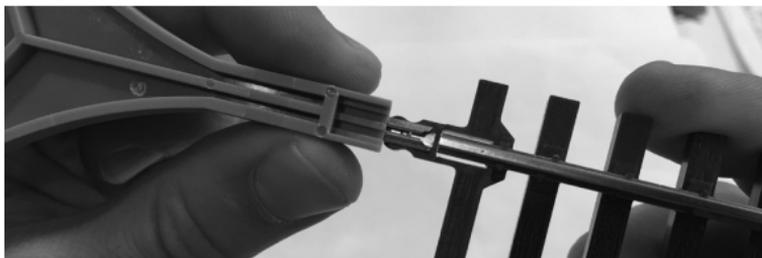
**Step 3** Use end of tool to affix rail joiner fully onto track.
