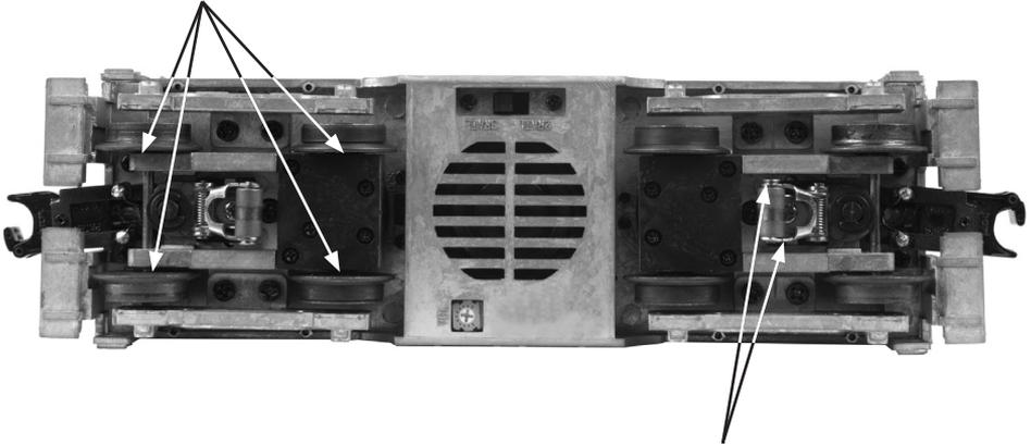
**Lubricate All Pick Up Roller Axles (L)**
