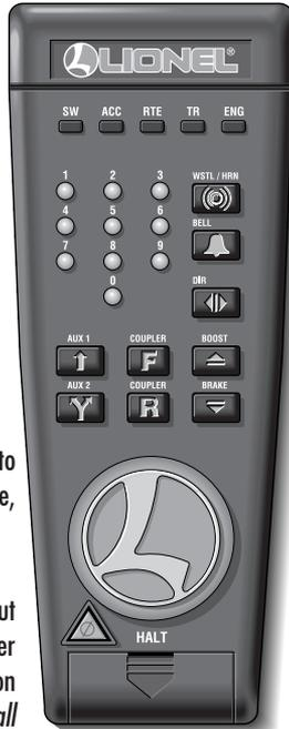
Press WSTL/HRN to activate the loco horn; release it to discontinue. **MultiHorn diesel horn sound.**
