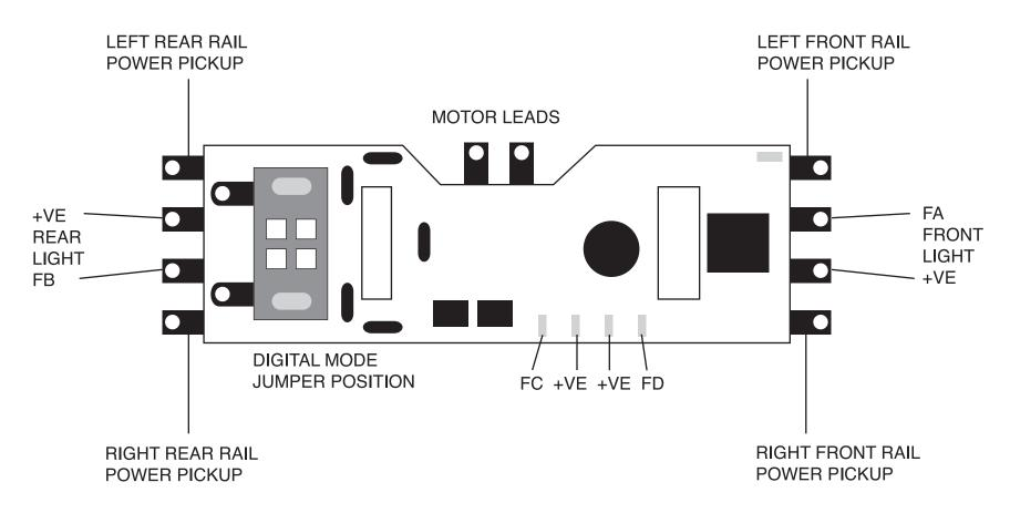
+VE IS THE POSITIVE COMMON RETURN LEAD FOR ALL FOUR FUNCTIONS - FA,FB,FC,FD
