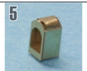
A photo of the completed signal head box. Strengthen the structure with small dabs of glue.
