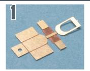
Remove all parts including the main piece (pictured) from the etching with sharp hobby knife.
