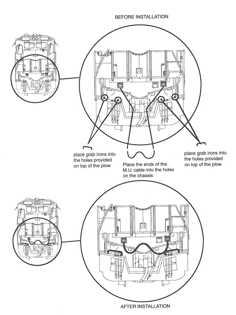
PLEASE NOTE: The M.U. cable may interfere with the snow plow on tight curvatures. This is not a problem on 2 rail version of the locomotive.
