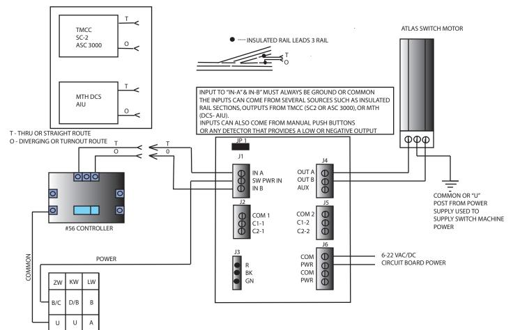
WIRING REQUIRED TO OPERATE ATLAS SWITCH MOTORS UTILIZING THE MANUAL #56 OR OTHER SIMILAR PUSH BUTTON ACTIVATION DEVICE. \* NOTE THE WIRING CHANGE FROM THE STANDARD INSTALLATION PROVIDED WITH THE DOCUMENTATION ENCLOSED WITH EVERY ATLAS SWITCH. WHEN USING THE UNIVERSAL SWITCH CONTROL CIRCUIT YOU MUST REWIRE ANY EXISTING INSTALLATION TO MATCH THIS SCHEMATIC.
