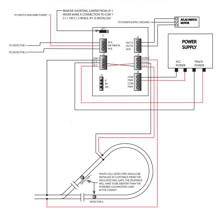
DETECTION FOR TWO RAIL APPLICATIONS WILL BE REQUIRED. THE ABOVE DIAGRAM SHOWS THE PLACEMENT FOR TWO PHOTO CELL DETECTORS. THE OUTPUT FROM THE DETECTORS WILL BE USED TO ACTIVATE THE USC BOARD. THE DETECTOR OUTPUTS WILL CONNECT TO THE USC CIRCUIT BOARD "IN A" AND "IN B"
