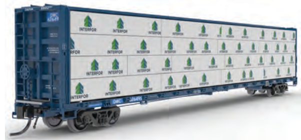
Artist rendering of the Canadian National 73' Center Divider Flat Car with separate sale load.
