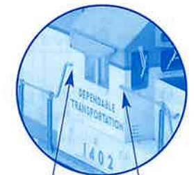
Carefully pull out handrails from the cab when removing body. The handrails are part of the chassis. Use a piece of paper or an index card to protect the body paint on the cab when removing the body.
